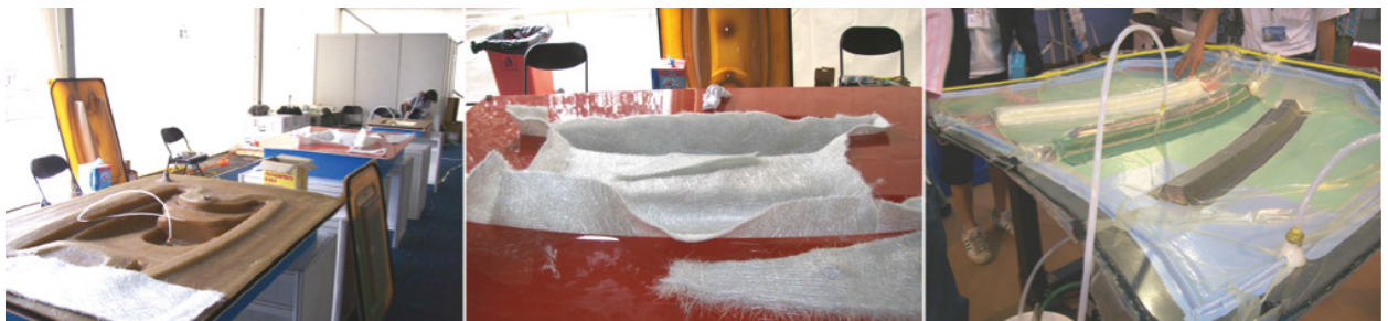
Photo 4. Vacuumed die molds for complex shape composite parts molding.
