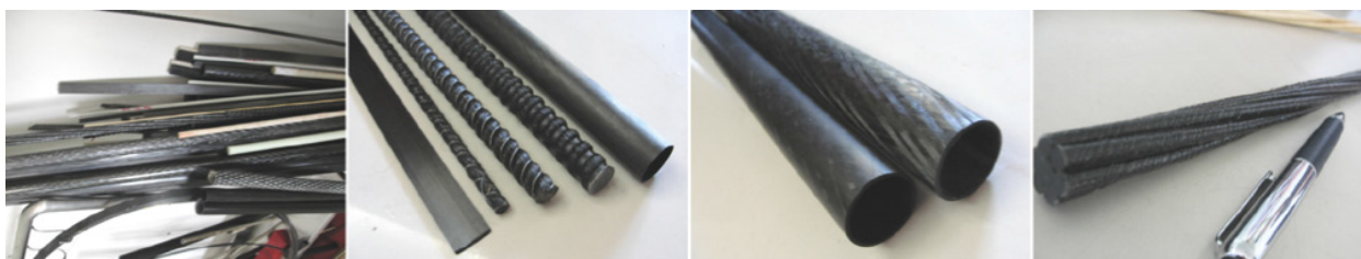
Photo 1. Longitudinal profile materials made of BCF roving, rebar, pipes, wire rope
