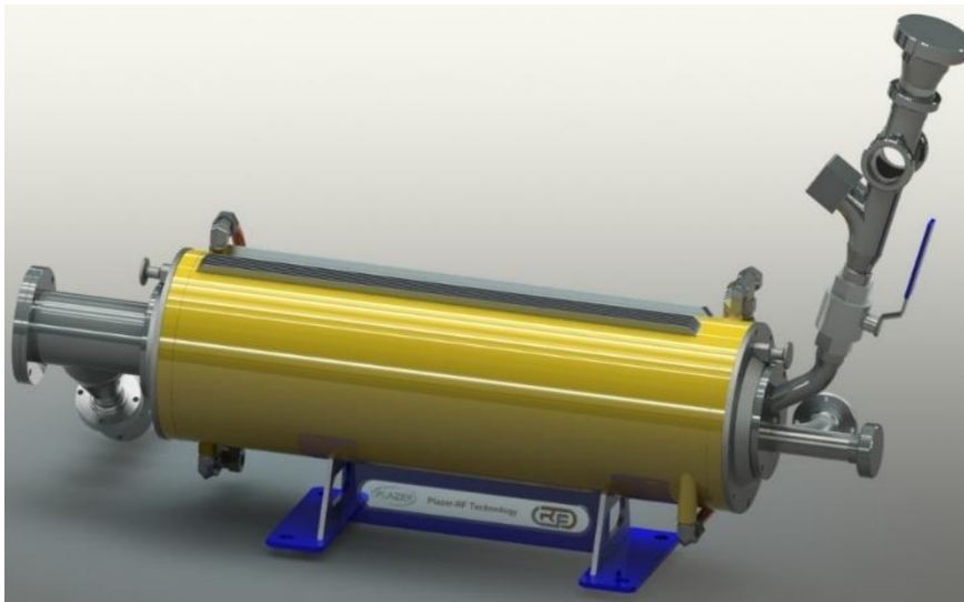
Fig. 2.1. The apparatus for microarc materials processing in the rotating electromagnetic field of the Plazer-RF
